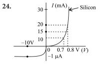
In diagram, At I = 20 mA, V = 0.8 V and At I = 10 mA, V = 0.7 V
