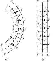
Huygens' geometrical construction for the propagation of (a) spherical, (b) plane wavefront.
